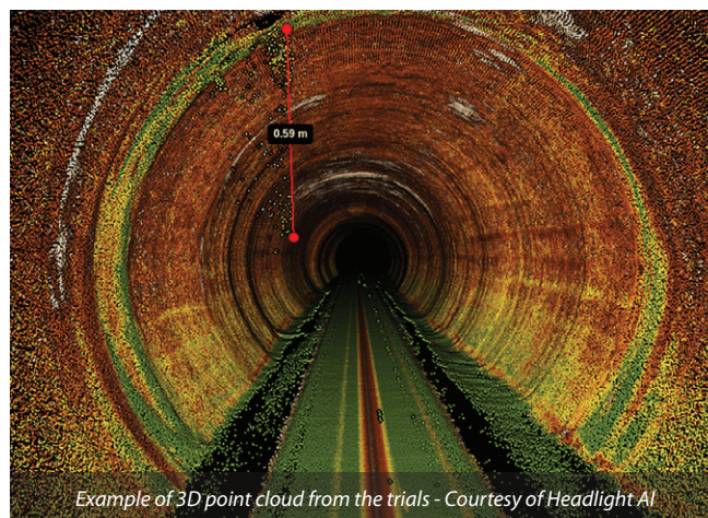
(top) Section of the sewer showing calcification and degradation and (below) the 3D point cloud at the same position - Courtesy of Headlight AI
