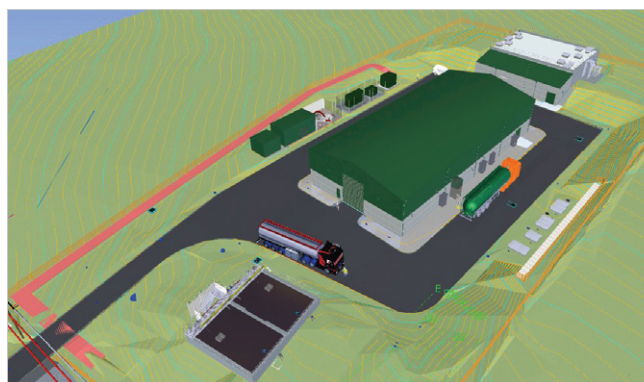
The Revit and Civils 3D models were combined to enable the landscaping, structural details and pipework to be accurately modelled Courtesy of MMB
