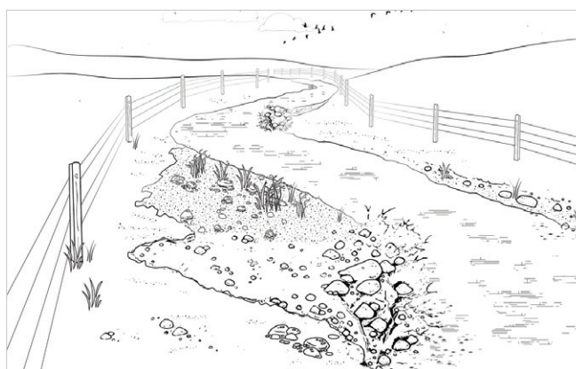
Figure 4: Indicative drawing of meandering river within its existing channel due to the installation of in-channel berms - Courtesy of Affinity Water
