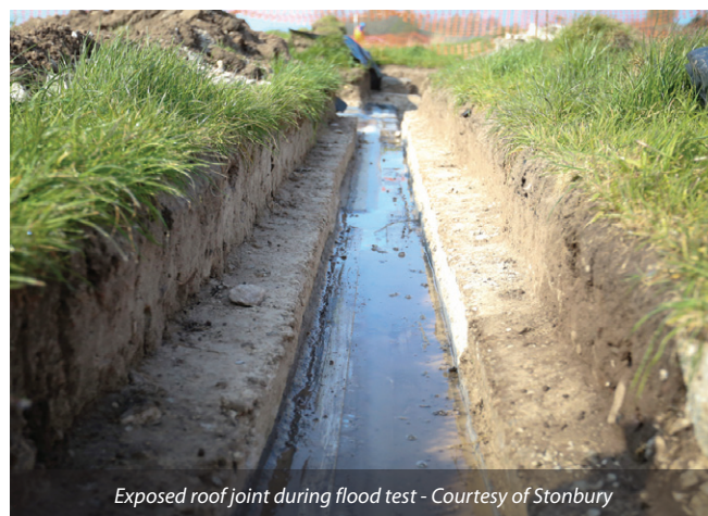
As directed by the client, specific sections of the roof were excavated, in preparation for the flood test - Courtesy of Stonbury
