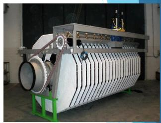
Tertiary Multi Disc Deep Pile Cloth Filters with 5 Micron Microfibre in a Stainless Steel Tank
