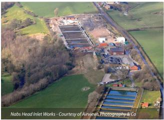
The works treats principally domestic crude sewage from the Blackburn catchment, with two major additional contributions; a high strength trade effluent from the brewery and an ammonia rich return liquor flow from the sludge treatment plant. The key river water quality/water framework directive parameters within the revised environmental permit are the need to achieve a BOD of 7mg/l and Ammonia of 1mg/l both on a 95%ile basis.
