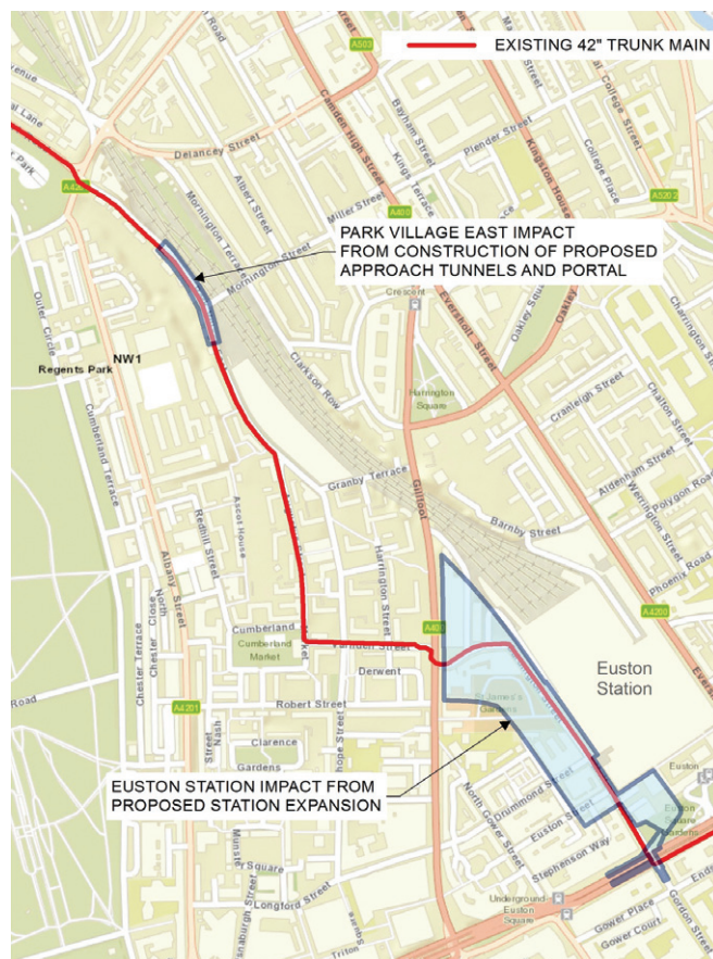
HS2 construction areas impacting the 42" trunk main (flow is north to south) - Courtesy of Stantec
