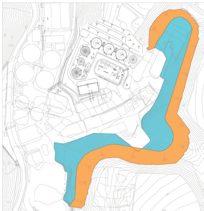
Figure 5: Plan showing extent of hillside removal and re-profiling in blue and the new slopes in orange - Courtesy of Sweco UK Ltd
