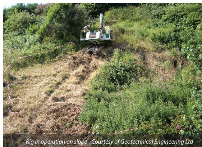
Slope climbing test rig for dynamic and rotary boring - Courtesy of aBV
