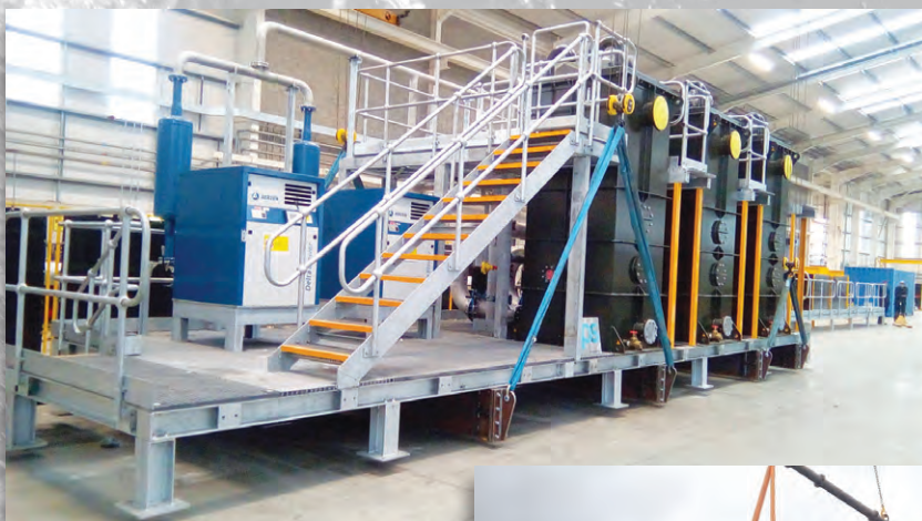
Tertiary treatment skid pre-assembled off-site - Courtesy of EPS
