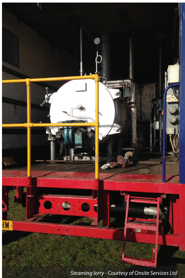
Curing the lining - Courtesy of Wessex Water
