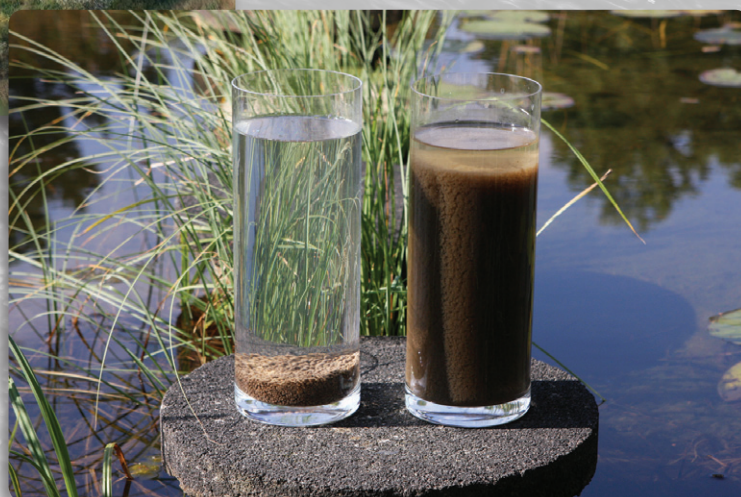
Settling Properties of the aerobic granular biomass (left) compared to activated sludge (right) Courtesy of Royal HaskoningDHV
