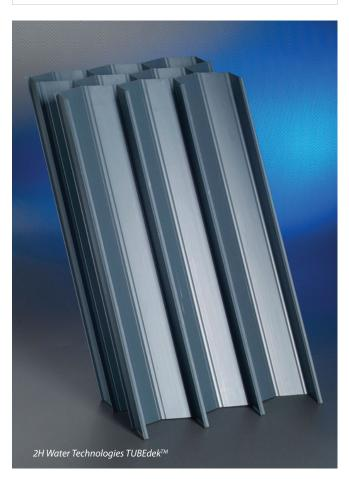
inclined angle of the tubes encourages laminar flow for efficient solids separation whilst the 'v' shape encourages a more even discharge of solids to the settlement zone below the  $TUBEdek^{TM}$  modules.
