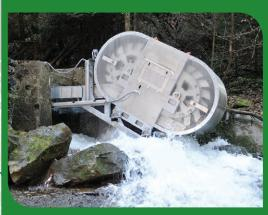
**STEFFTURBINE** – small scale micro hydroelectric turbine power plant rated to produce up to 12 kW LV power. Uses mainly potential energy to drive conveyor based turbine generator. Two sizes; 250-400 l/s (requiring 3.5-5.0 m available head) & 400-600 l/s (requiring 2.0-3.5m available head). Efficiencies beteen 70-90% expected depending on application. Contact Sewaco for more information.
