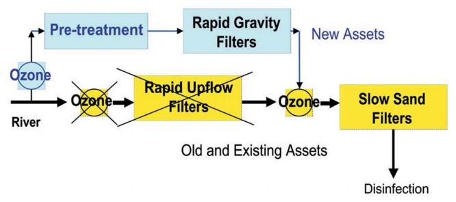
Schematic showing Fobney WTW Process Upgrade
