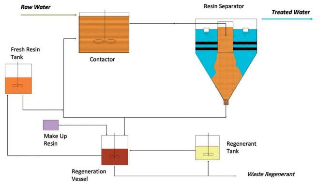
Process Flow diagram of the MIEX® Process
